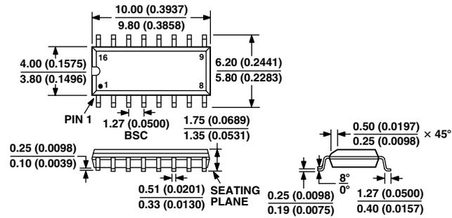
CONTROLLING DIMENSIONS ARE IN MILLIMETERS; INCH DIMENSIONS (IN PARENTHESES) ARE ROUNDED-OFF MILLIMETER EQUIVALENTS FOR REFERENCE ONLY AND ARE NOT APPROPRIATE FOR USE IN DESIGN
