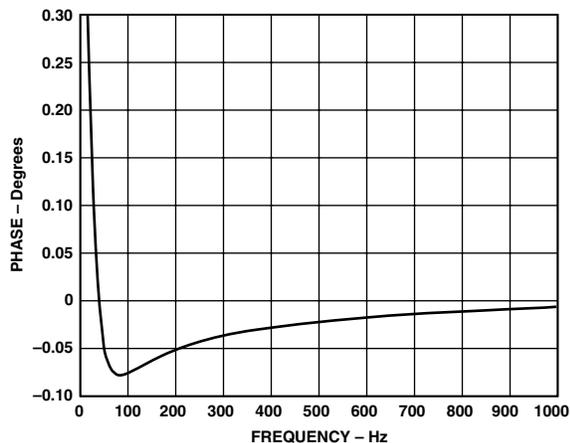
Figure 11. Phase Error between Channels (0 Hz to 1 kHz)
