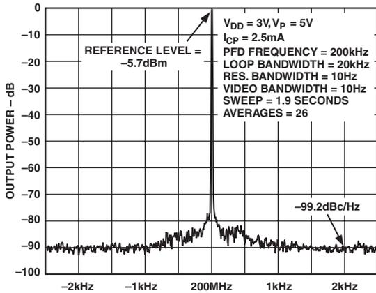
TPC 3. Phase Noise (200 MHz, 200 kHz, 20 kHz)
