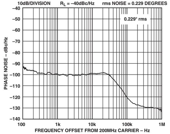
TPC 4. Integrated Phase Noise (200 MHz, 200 kHz, 20 kHz)
