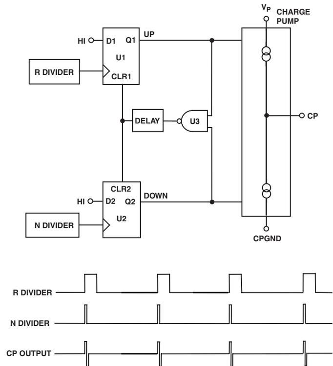
Figure 5. PFD Simplified Schematic and Timing (In Lock)
