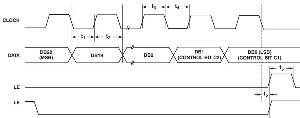
Figure 1. Timing Diagram
