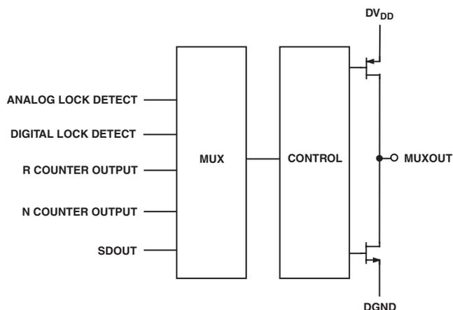
Figure 6. MUXOUT Circuit
