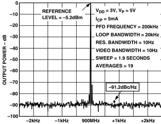
TPC 2. ADF4213 Phase Noise (900 MHz, 200 kHz, 20 kHz)
