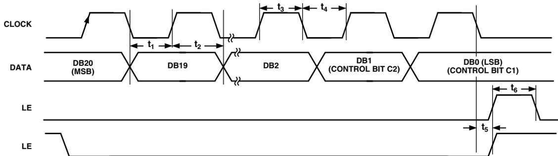
Figure 1. Timing Diagram
