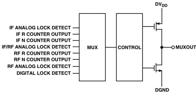
Figure 6. MUXOUT Circuit
