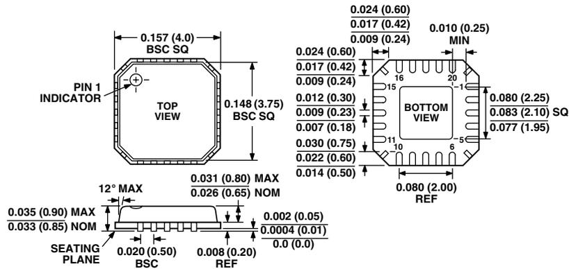
CONTROLLING DIMENSIONS ARE IN MILLIMETERS
