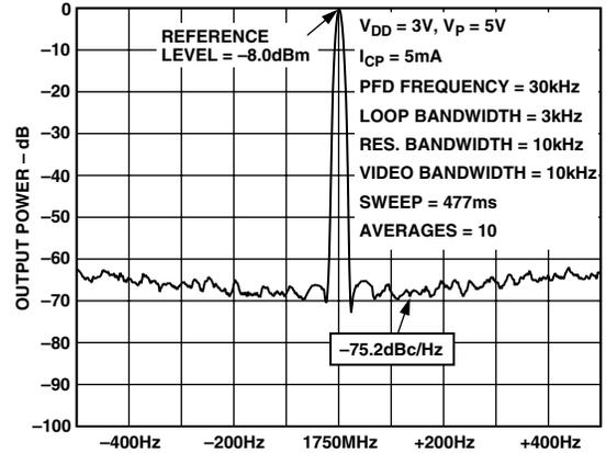
TPC 10. ADF4213 Phase Noise (1750 MHz, 30 kHz, 3 kHz)
