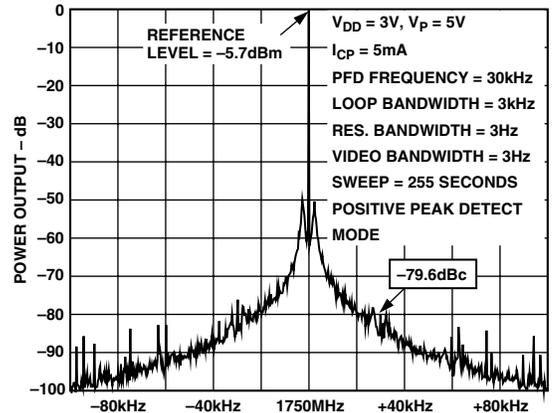
TPC 11. ADF4213 Reference Spurs (1750 MHz, 30 kHz, 3 kHz)
