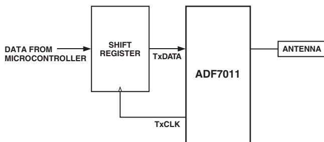
Figure 14. TxCLK Pin Synchronizing Data for GFSK
