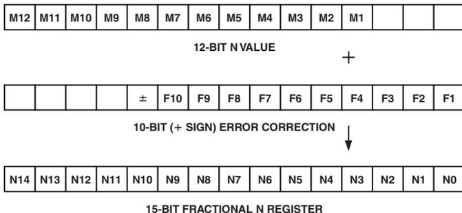
Figure 12. Fractional Components
