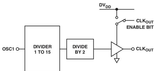
Figure 3. CLK<sub>OUT</sub> Stage
