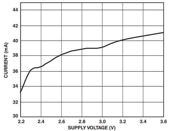
TPC 12.  $I_{DD}$  vs.  $V_{DD}$  @ 10 dBm
