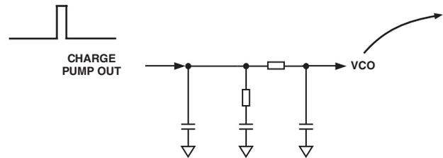
Figure 6. Typical Loop Filter Configuration—Third Order Integrator
