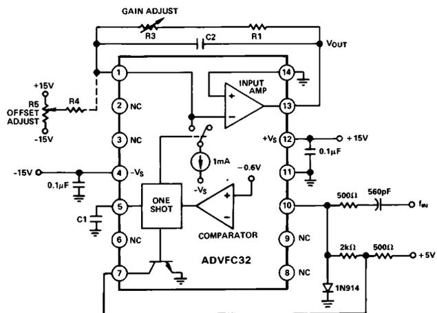
Figure 4. Connection Diagram for F/V Conversion, TTL Input
