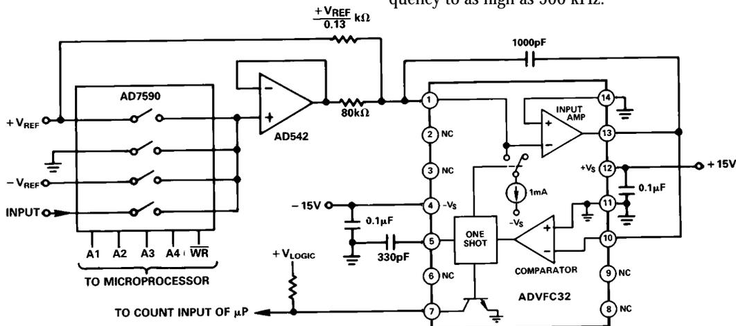
Figure 5. High Resolution, Self-Calibrating, Microprocessor Operated A/D Converter
