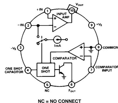
2. The ADVFC32 is easily configured to satisfy a wide range of system requirements. Input voltage scaling is set by selecting the input resistor which sets the input current to 0.25 mA at the maximum input voltage.
