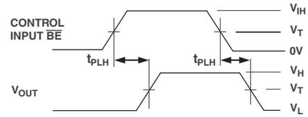
Figure 2. Propagation Delay
