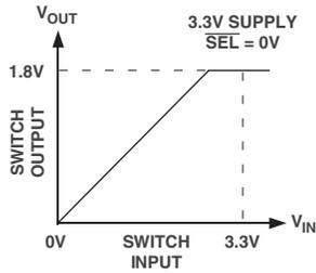
Figure 10. 3.3 V to 1.8 V Voltage Translation,  $\overline{SEL} = 0 V$
