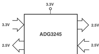
Figure 5. 3.3 V to 2.5 V Voltage Translation,  $\overline{SEL} = V_{CC}$
