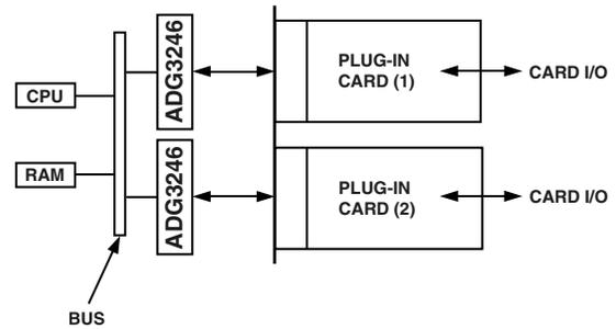
Figure 12. ADG3246 in a Hot Plug Application
