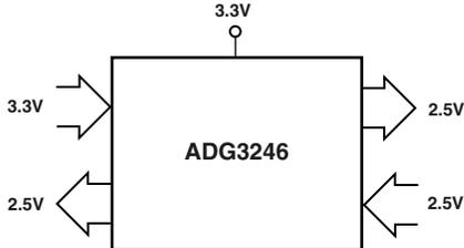
Figure 5. 3.3 V to 2.5 V Voltage Translation,  $\overline{SEL} = V_{CC}$
