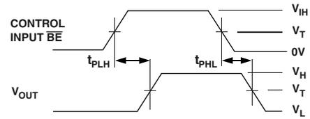
Figure 2. Propagation Delay
