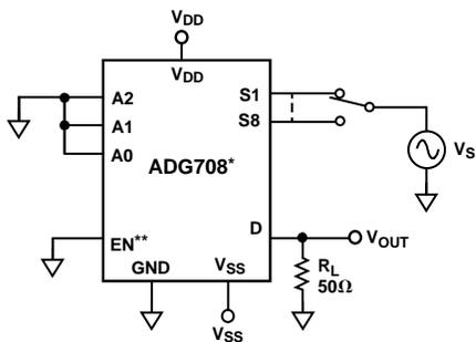
$$\text{OFF ISOLATION} = 20\text{LOG}_{10} \frac{V_{\text{OUT}}}{V_{\text{S}}}$$
