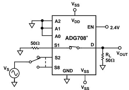
$$\text{CHANNEL-TO-CHANNEL CROSSTALK} = 20\text{LOG}_{10} \frac{V_{\text{OUT}}}{V_{\text{S}}}$$
