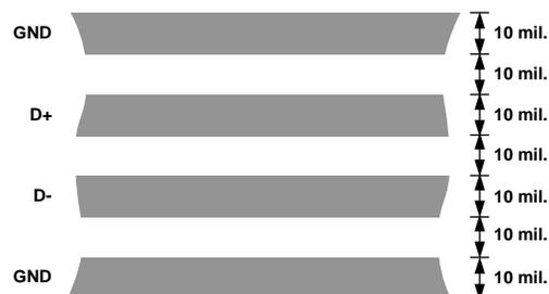
Figure 17. Arrangement of Signal Tracks
