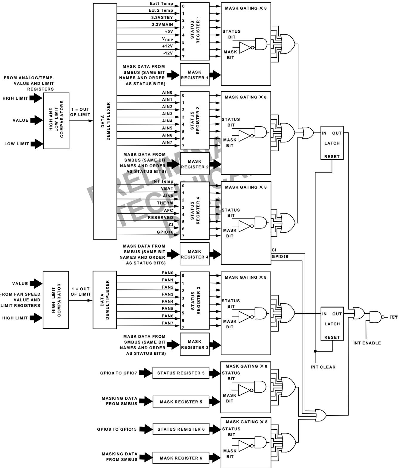
Figure 15. ADM1026 Interrupt Structure
