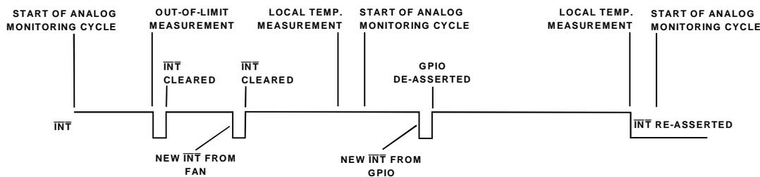
Figure 17. Other Interrupt Sources Can Re-assert INT Immediately
