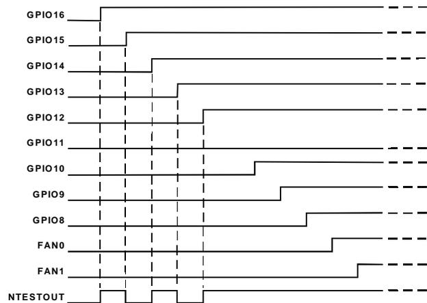
Figure 24. NAND Tree Test With GPIO11 Stuck Low
