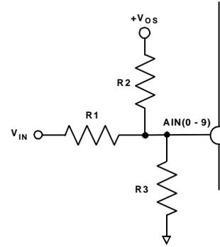
Figure 7. Scaling and Offsetting AIN(0 - 9) for Bipolar Inputs
