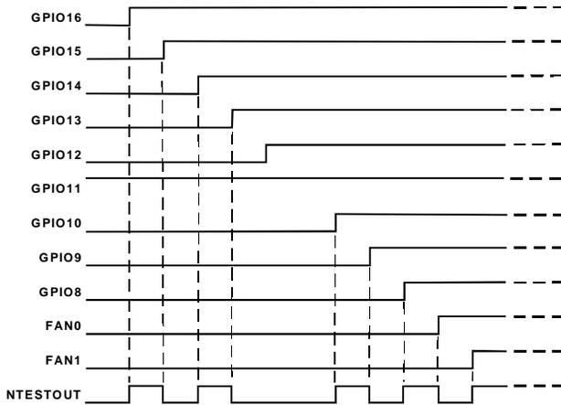
Figure 25. NAND Tree Test With One Input Stuck High
