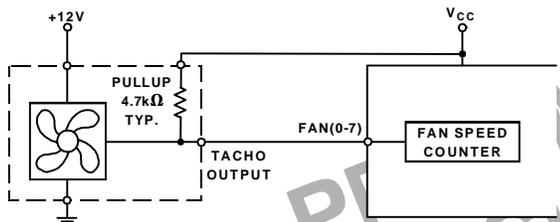
Figure 12a. Fan With Tach Pullup To + $V_{CC}$ .
