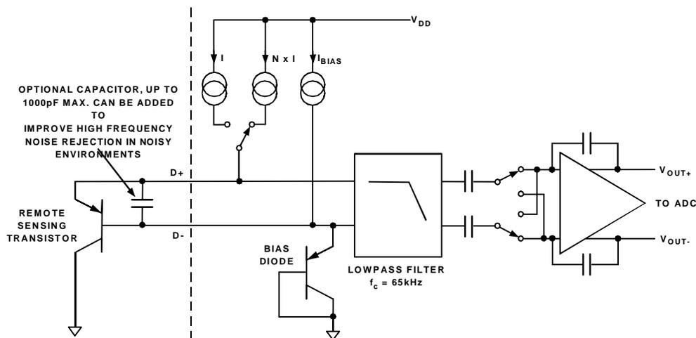
Figure 8. Signal Conditioning for Remote Diode temperature Sensors
