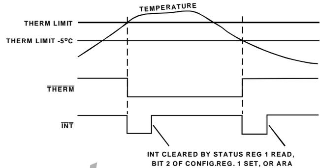
Figure 19. Assertion Of  $\overline{INT}$  Due To  $\overline{THERM}$  Event
