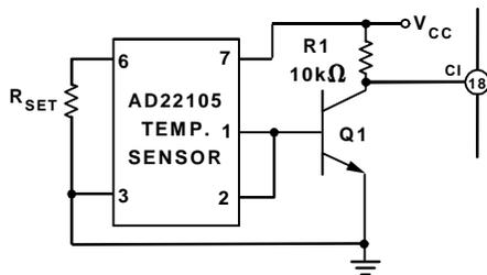
Figure 14. Using the CI Input with a Temperature Sensor
