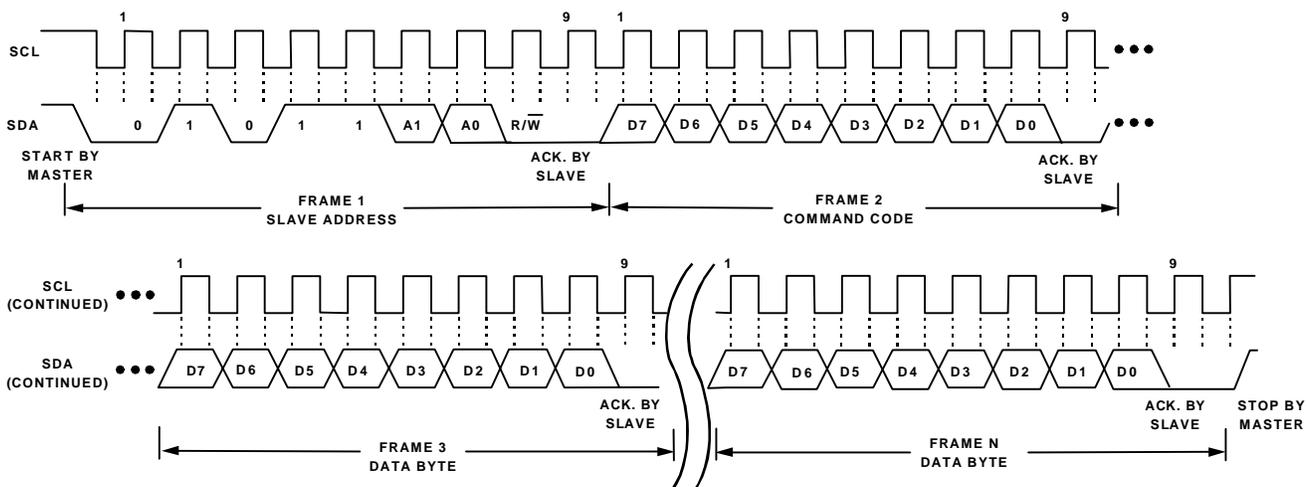
Figure 2a. General SMBus Write Timing Diagram
