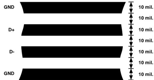
Figure 9. Arrangement of Signal Tracks
