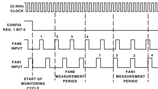
Figure 13. Fan Speed Measurement
