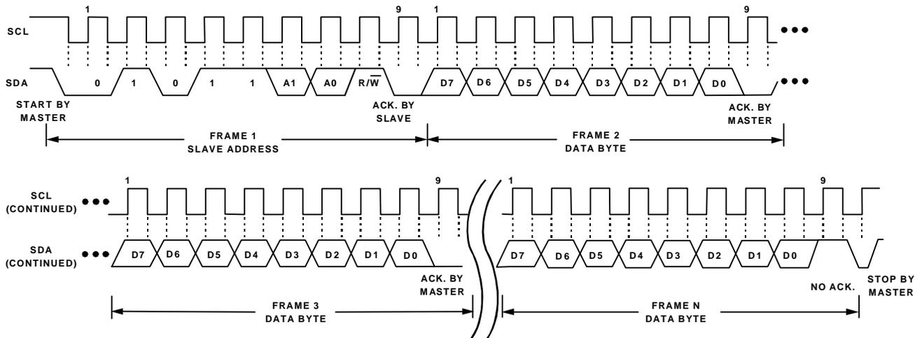
Figure 2b. General SMBus Read Timing Diagram
