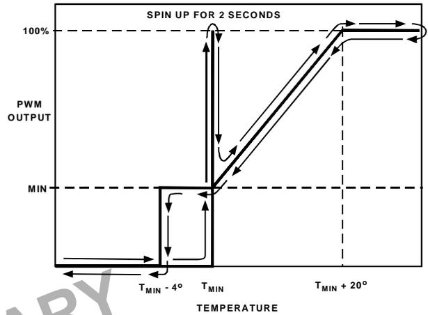
Figure 11a. Automatic PWM Fan Control Transfer Function
