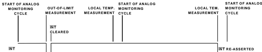
Figure 16. Delay After Clearing INT Before Re-assertion
