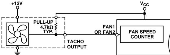
Figure 6a. Fan with Tachometer Pull-Up to  $+V_{CC}$
