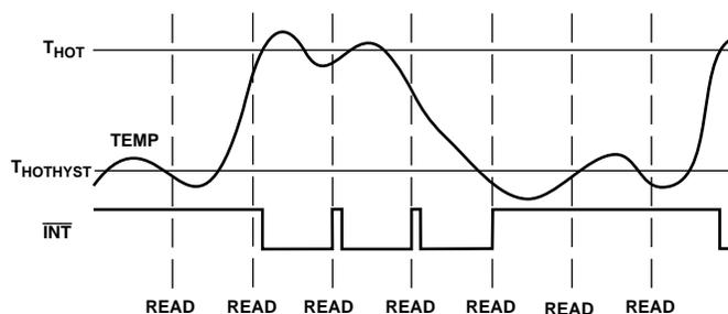
Figure 10. Temperature  $\overline{\text{INT}}$  Output in Default Interrupt Mode
