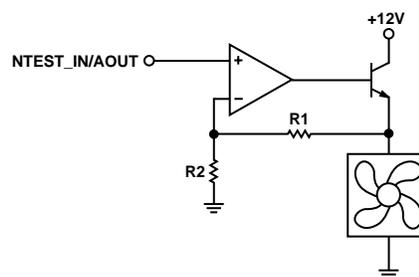
Figure 5. Analog Output Driving Fan
