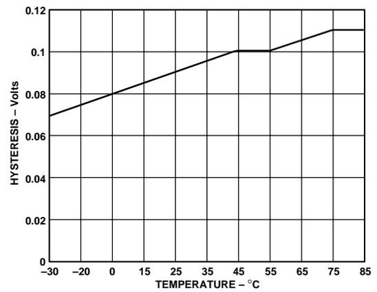
Figure 5. Hysteresis vs. Temperature for SU3—Low to High
