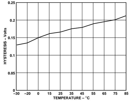
Figure 4. Hysteresis vs. Temperature for SU2—High to Low
