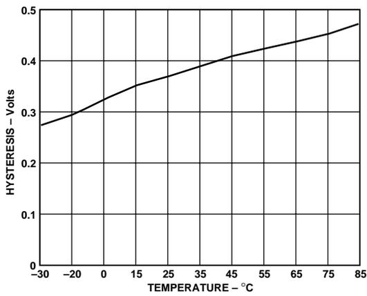
Figure 2. Hysteresis vs. Temperature for SU1—High to Low
