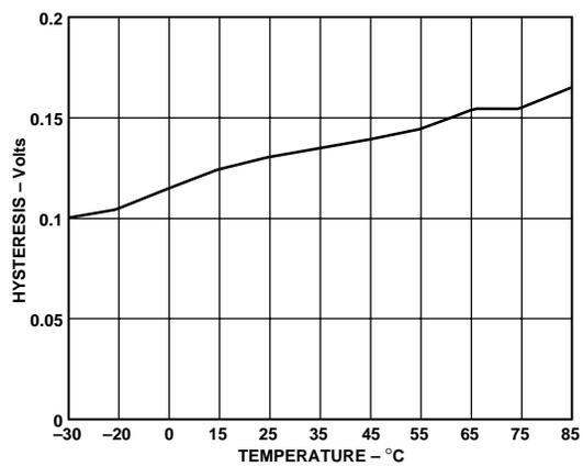
Figure 3. Hysteresis vs. Temperature for SU2—Low to High
