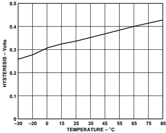
Figure 1. Hysteresis vs. Temperature for SU1—Low to High
