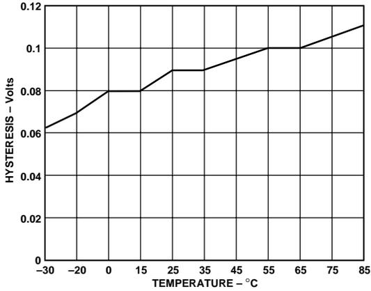
Figure 8. Hysteresis vs. Temperature for SU4—High to Low
