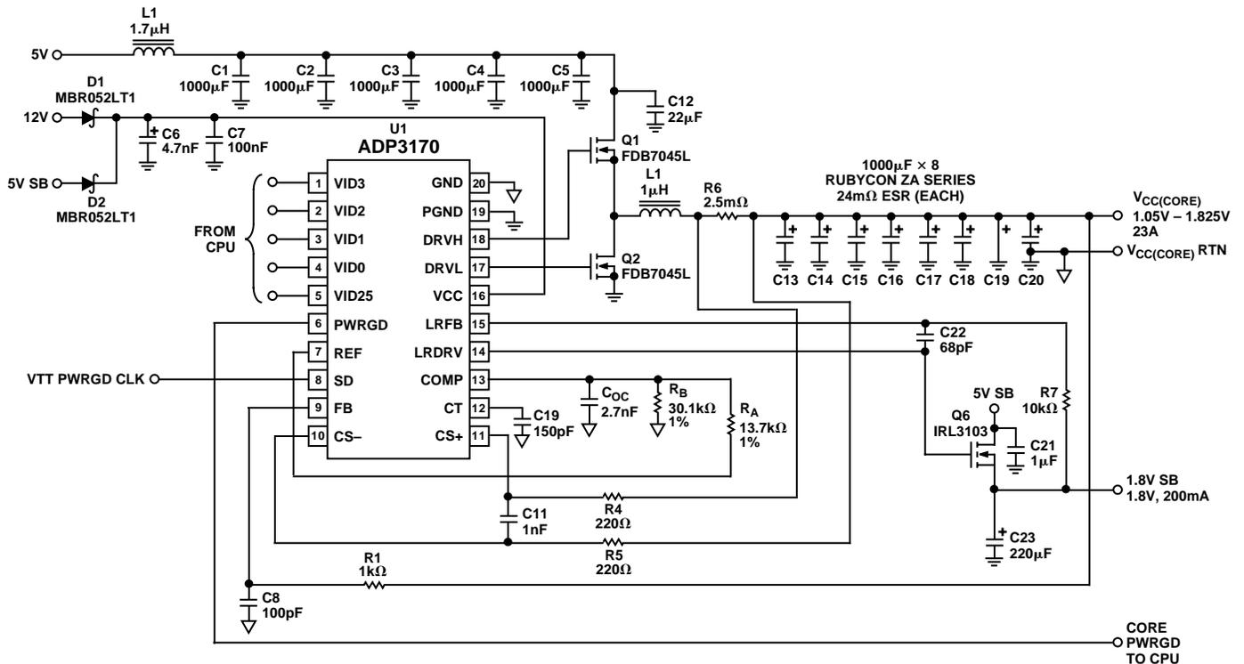
*Figure 3. 24 A VRM 8.5-Compliant CPU Supply*
