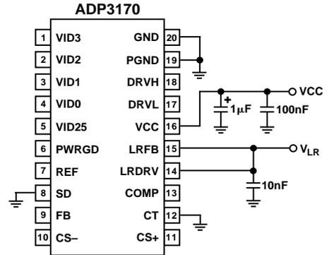
Figure 2. Linear Regulator Output Voltage Accuracy Test Circuit
