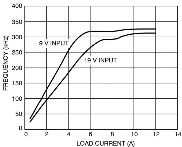
**Figure 28. Single-Phase CCM/DCM Frequency vs. Load Current**
