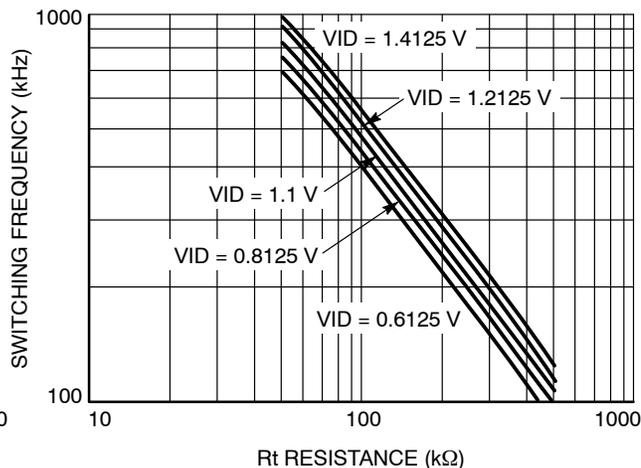
**Figure 7. Per Phase Switching Frequency vs. RT Resistance**
