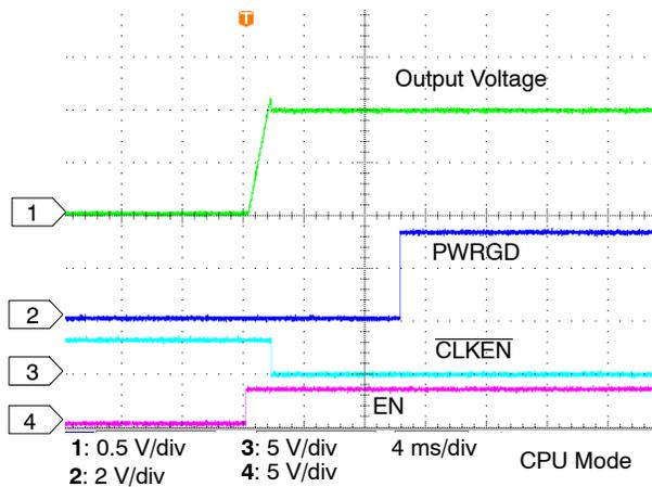
**Figure 9. Startup in CPU Mode**
