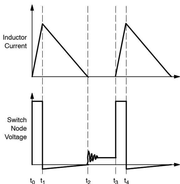
**Figure 26. Inductor Current and Switch Node in DCM**
