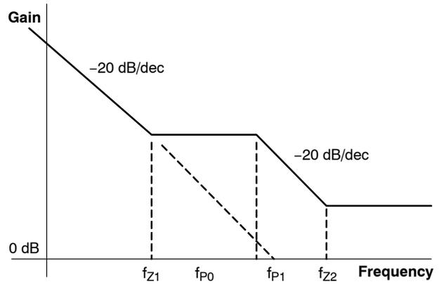
Figure 32. Poles and Zeros of Voltage Error Amplifier
