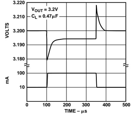
Figure 13. Load Transient
