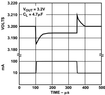
Figure 14. Load Transient
