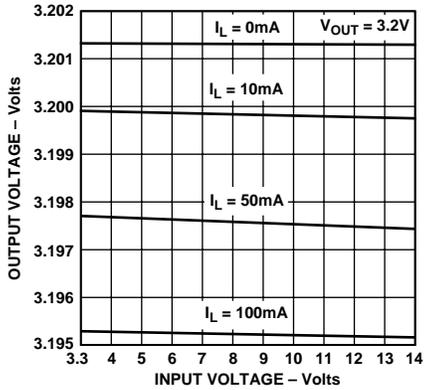
Figure 2. Line Regulation Output Voltage vs. Supply Voltage
