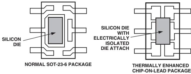
Figure 4. Chip-on-Lead Package
