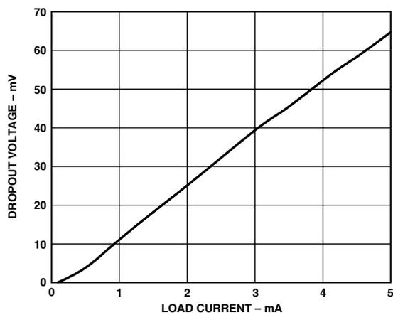
TPC 3. VTCXO Dropout Voltage vs. Load Current
