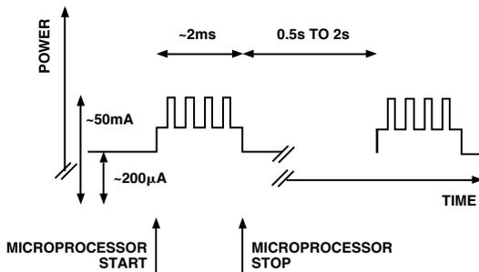
Figure 4. Digital Power as a Function of Time
