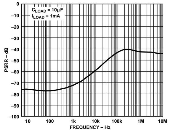
Figure 12. Ripple Rejection\*
