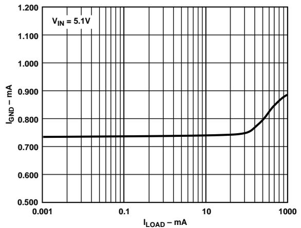
Figure 7.  $I_{GND}$  vs.  $I_{LOAD}$  ( $V_{IN} = 5.1 V$ )\*
