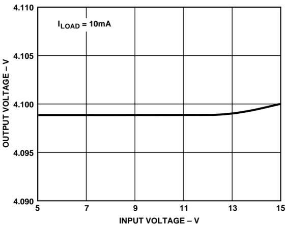
Figure 4.  $V_{OUT}$  vs.  $V_{IN}$  ( $I_{LOAD} = 10 mA$ )\*
