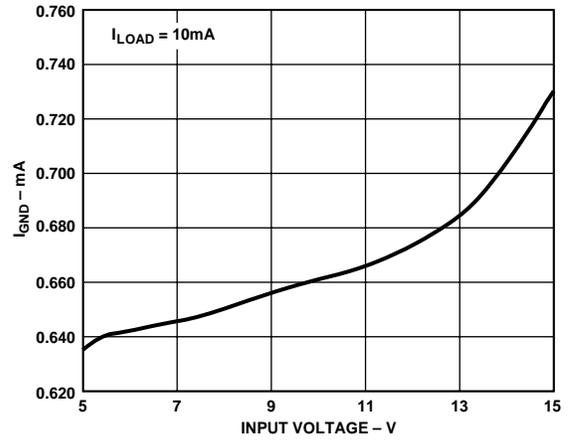
Figure 5.  $I_{GND}$  vs.  $V_{IN}$  ( $I_{LOAD} = 10 mA$ )\*
