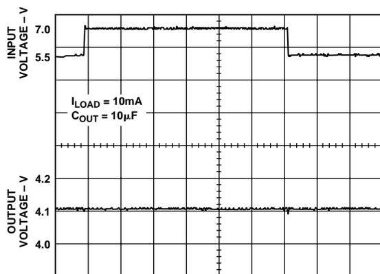
Figure 10. Line Transient Response ( $10\mu F$  Output Cap)\*
