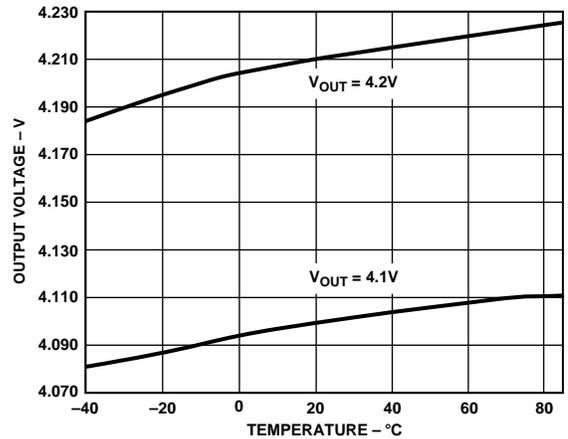
Figure 11.  $V_{OUT}$  vs. Temperature,  $V_{IN} = 5.1V$ ,  $I_{LOAD} = 10mA$ \*
