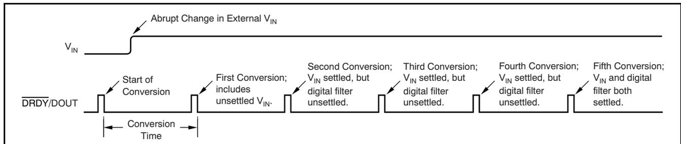
Figure 5. Settling Time in Continuous Conversion Mode
