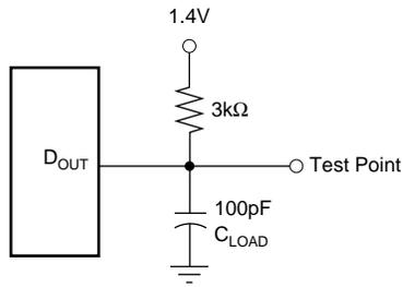
Load Circuit for  $t_{dDO}$ ,  $t_r$ , and  $t_f$
