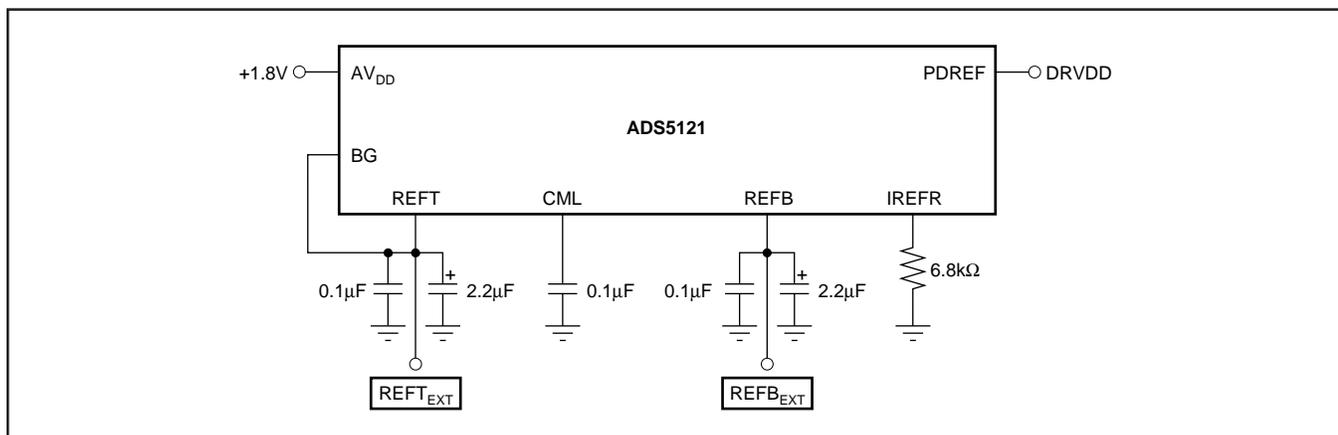
FIGURE 5. External Reference; Recommended Configuration and Bypassing.
