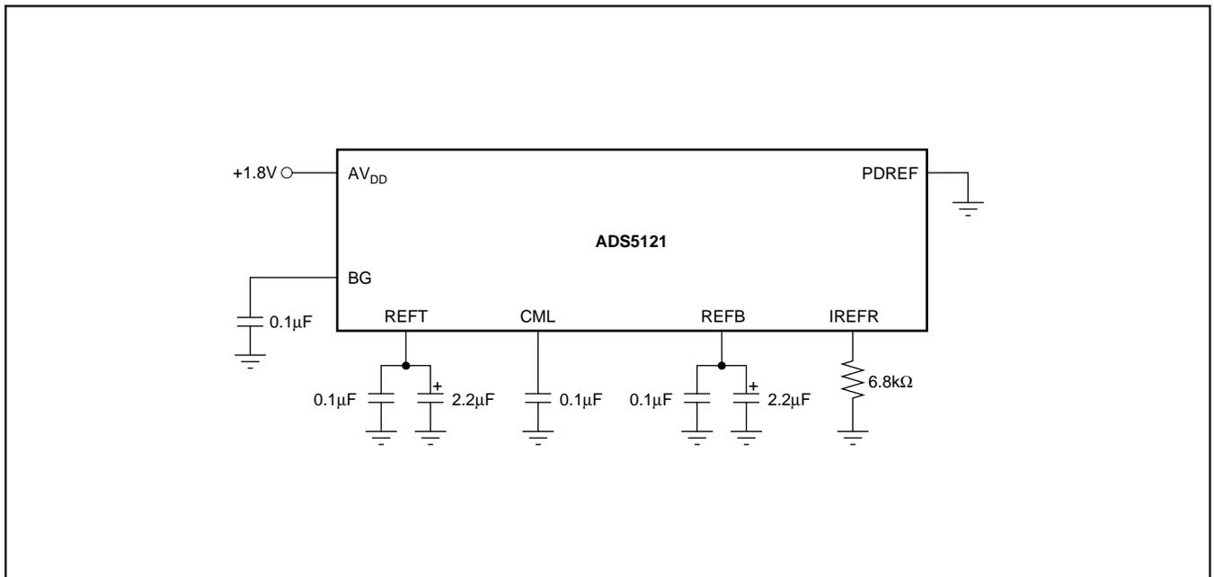
FIGURE 4. Internal Reference; Recommended Configuration and Bypassing.
