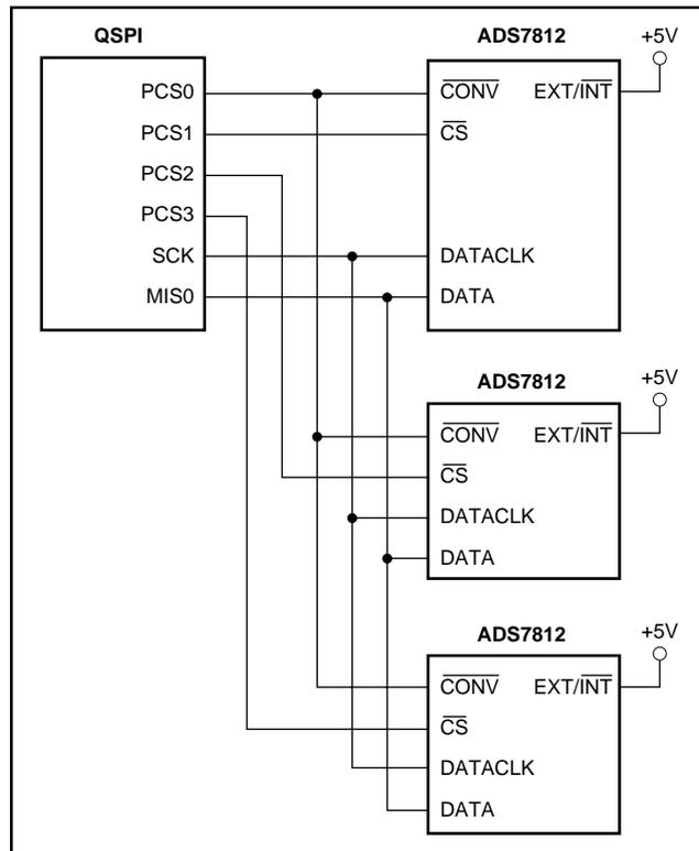
FIGURE 15. QSPI Interface to the Three ADS7812s.
