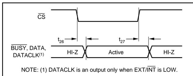
FIGURE 9. Enable and Disable Timing for Digital Outputs.
