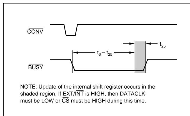
FIGURE 4. Timing of the Shift Register Update.
