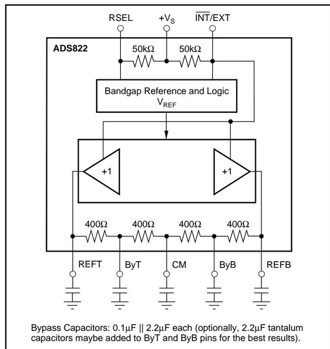
FIGURE 6. Equivalent Reference Circuit with Recommended Reference Bypassing.
