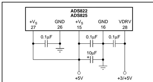
FIGURE 9. Recommended Bypassing for the Supply Pins.
