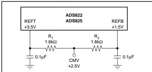
FIGURE 7. Alternative Circuit to Generate CM Voltage.
