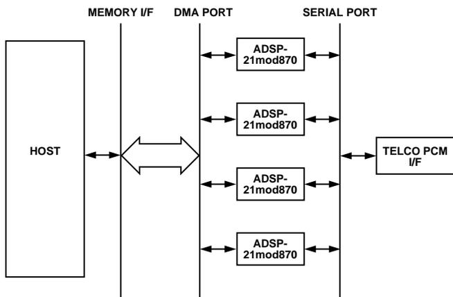
Figure 2. Serial Telco PCM TDM Data Stream Architecture
