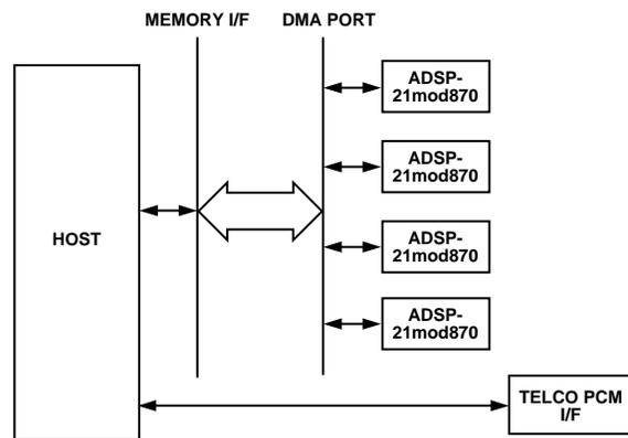
Figure 3. Parallel Telco PCM Data Stream Architecture
