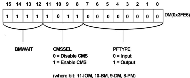
Figure 7. Programmable Flag<sup>1</sup> & Composite Select Control Register
