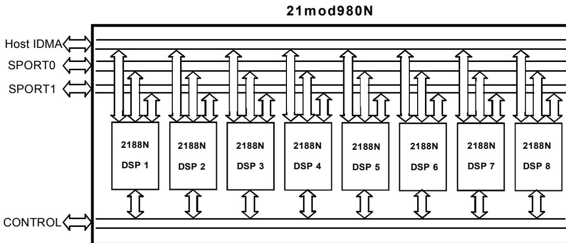
Figure 1. MOD980N MultiPort Internet Gateway Processor Block Diagram
