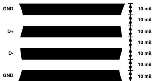
Figure 19. Arrangement of Signal Tracks
