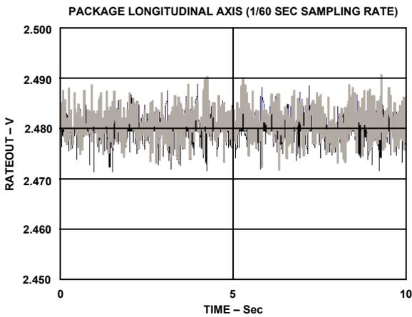
Figure 10. 10 g Random Vibration in Package-Longitudinal Axis Orientation
