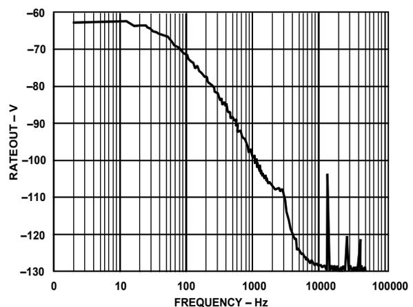
Figure 26. Noise Spectral Density at RATEOUT - BW = 4Hz
