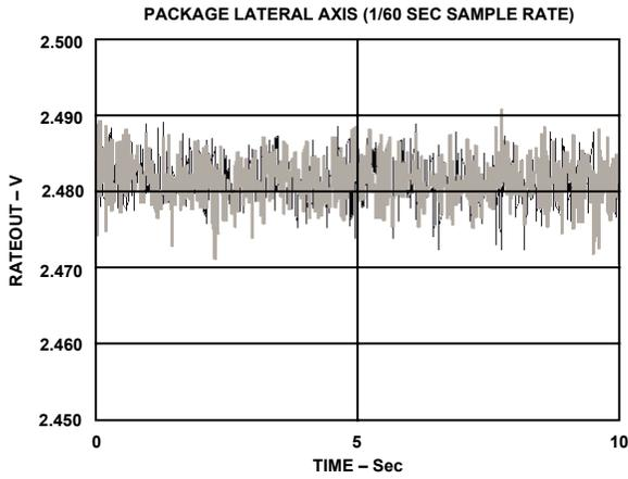
Figure 9. 10 g Random Vibration in Package-Lateral Axis Orientation
