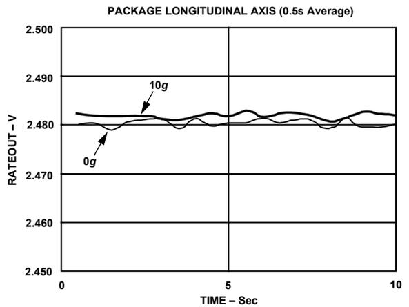
Figure 13. 10 g Random Vibration in Package-Longitudinal Axis Orientation
