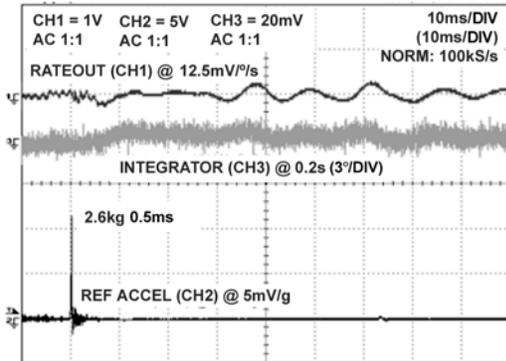
Figure 16. Hi-g Shock Test in Lateral Axis (40 Hz)
