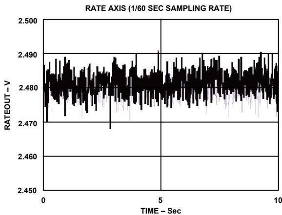
Figure 11. 10 g Random Vibration in Rate Axis Orientation
