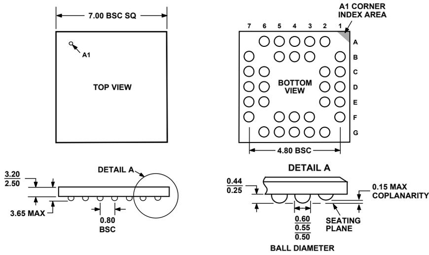
Figure 28. 32-Lead Chip Scale Ball Grid Array [CSPBGA]
