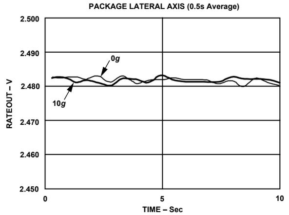
Figure 12. 10 g Random Vibration in Package-Lateral Axis Orientation
