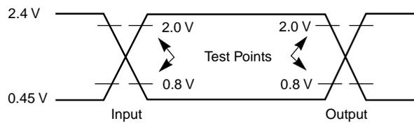
AC Testing (except for -55 devices): Inputs are driven at 2.4 V for a logic "1" and 0.45 V for a logic "0". Input pulse rise and fall times are  $\leq 20 \text{ ns}$ .
