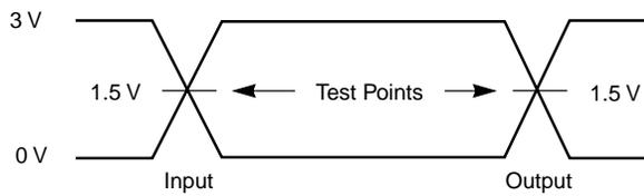
AC Testing for -55 devices: Inputs are driven at 3.0 V for a logic "1" and 0 V for a logic "0". Input pulse rise and fall times are  $\leq 20 \text{ ns}$ .
