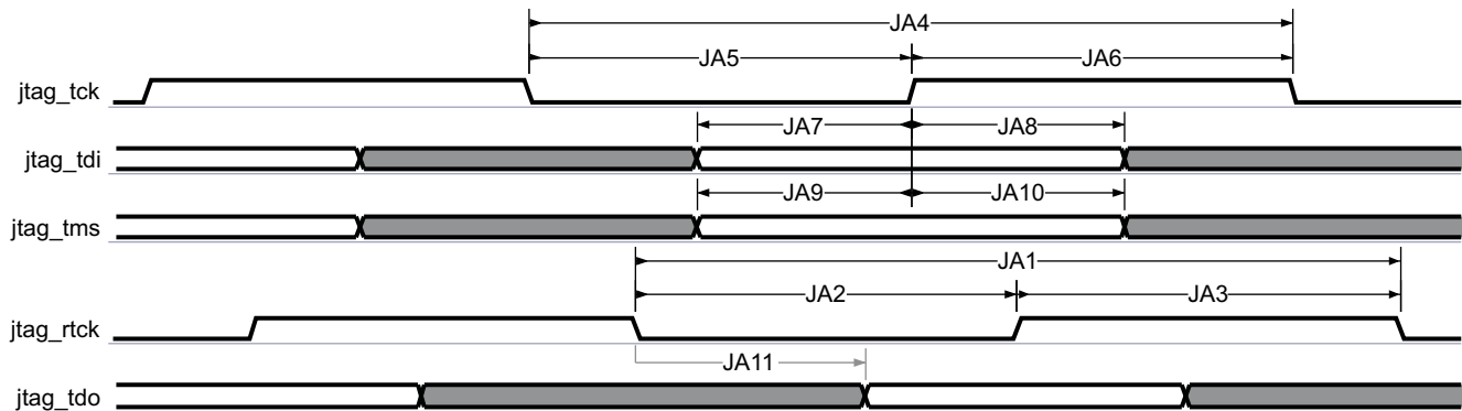
Figure 6-83. JTAG—Adaptative Clock Mode
