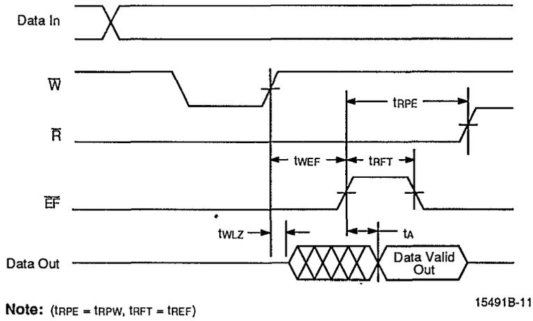
Figure 8. Read Data Flow-Through Mode
