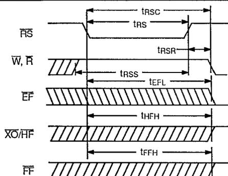
Figure 2. Reset Timing
