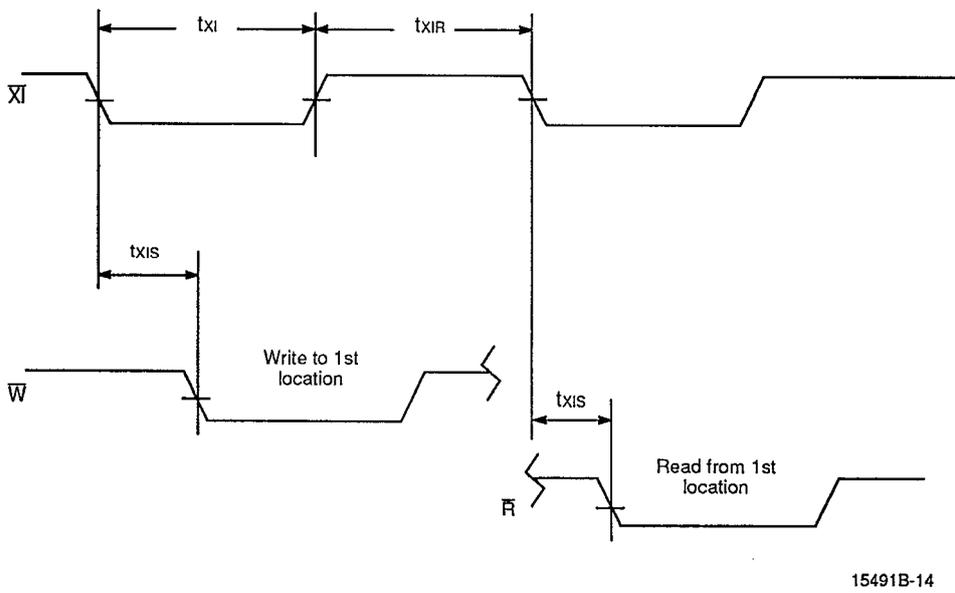
Figure 11. 1st Clock Pulse Delay from  $\overline{X1}$
