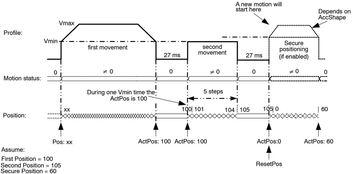
**Figure 8. Dual Positioning**
