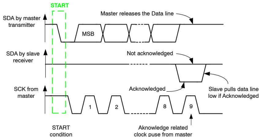
**Figure 26. Acknowledge on the I<sup>2</sup>C-bus**
