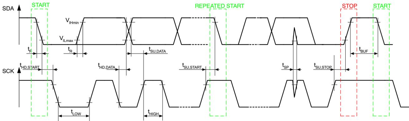
Figure 5. I<sup>2</sup>C Timing Diagrams
