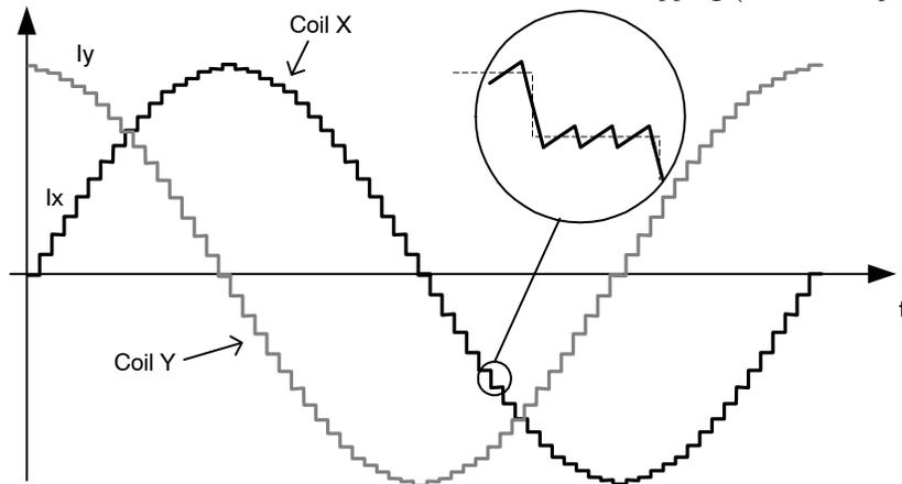
**Figure 19. Current Waveforms in Motor Coils X and Y in 1/16<sup>th</sup> Micro-Step Mode**
