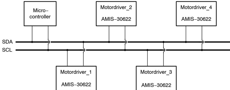
**Figure 21. Example of an I<sup>2</sup>C-bus Configuration Using One Microcontroller and Four Slaves**
