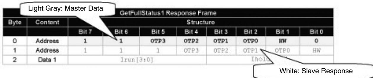
**Figure 33. Color Code Used in the Definition of I<sup>2</sup>C Frames**
