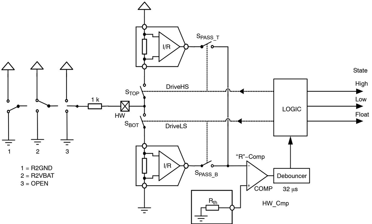
**Figure 10. Simplified Schematic Diagram of the HW Comparator**
