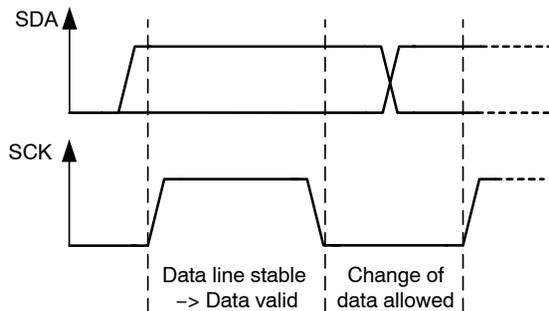
Figure 23. Bit Transfer on the I<sup>2</sup>C-bus
