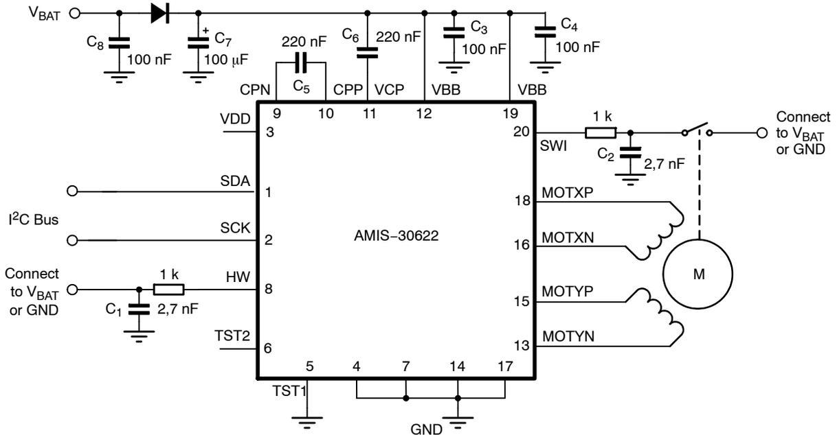
**Figure 6. Typical Application Diagram for SO Device**
