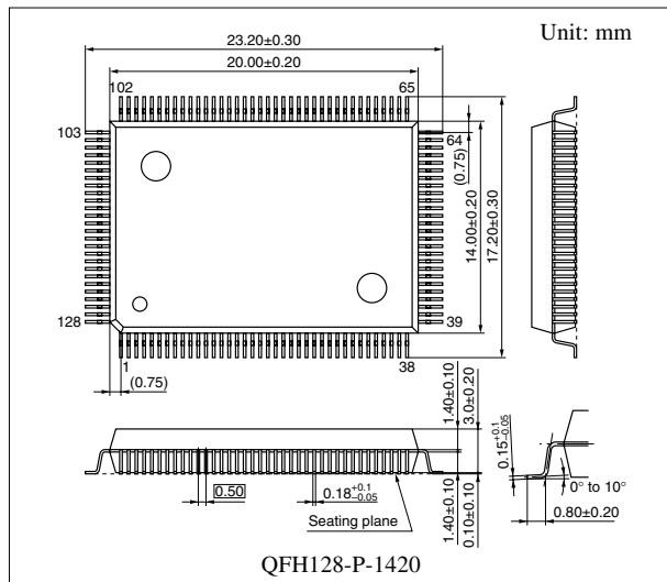
Note) The package of this product will be changed to lead-free type (QFH128-P-1420E). See the new package dimensions section later of this datasheet.
