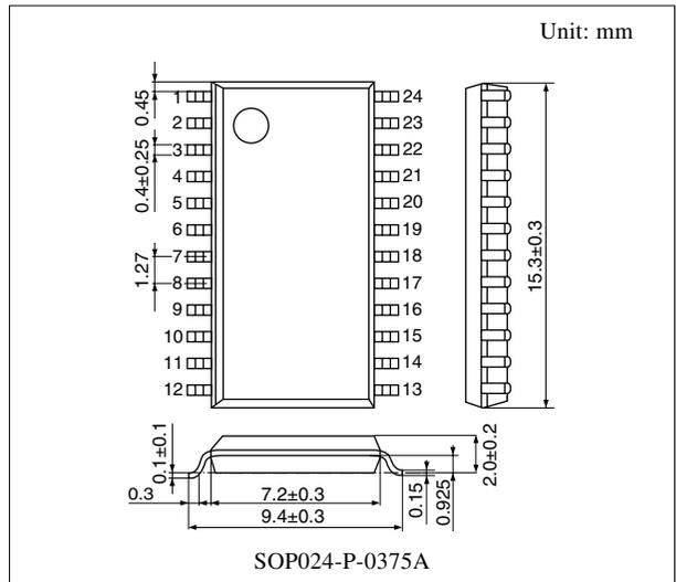
Note) The package of this product will be changed to lead-free type (SOP024-P-0375C). See the new package dimensions section later of this datasheet.
