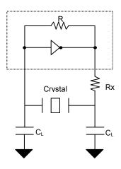
$$\begin{split} C_\text{L} &= 2^*(C_\text{P} - C_\text{S}), \\ \text{Where } C_\text{P} &= \text{Load capacitance of crystal} \\ C_\text{S} &= \text{Stray capacitance due to } C_\text{IN,} \text{ PCB, Trace etc.} \end{split}$$
