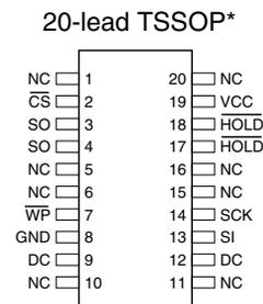
Note: \*Pins 3, 4 and 17, 18 are internally connected for 14-lead TSSOP socket compatibility.
