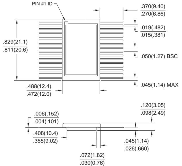
**32L**, 32-Pad, Non-Windowed, Ceramic Leadless Chip Carrier (LCC)
