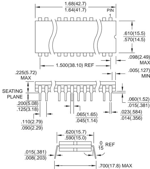
**32F**, 32-Lead, Non-Windowed, Ceramic Bottom Brazed Flat Package (Flatpack)
