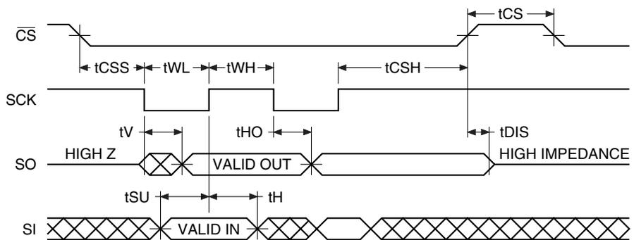
**Reset Timing (Inactive Clock Polarity Low Shown)**
