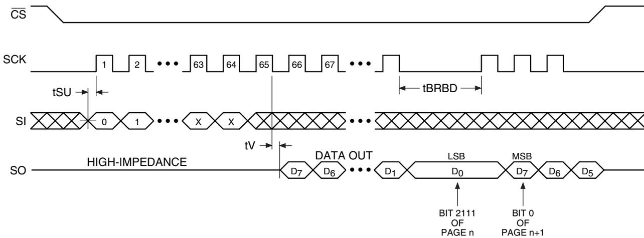
Detailed Bit-level Read Timing – Inactive Clock Polarity Low (Continued)
