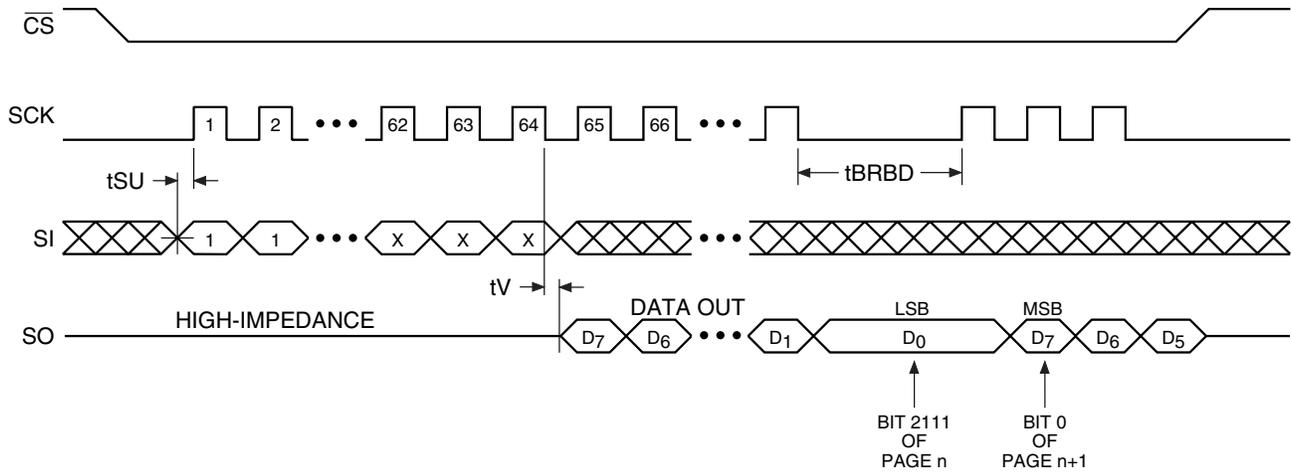
Detailed Bit-level Read Timing – SPI Mode 0 (Continued)
