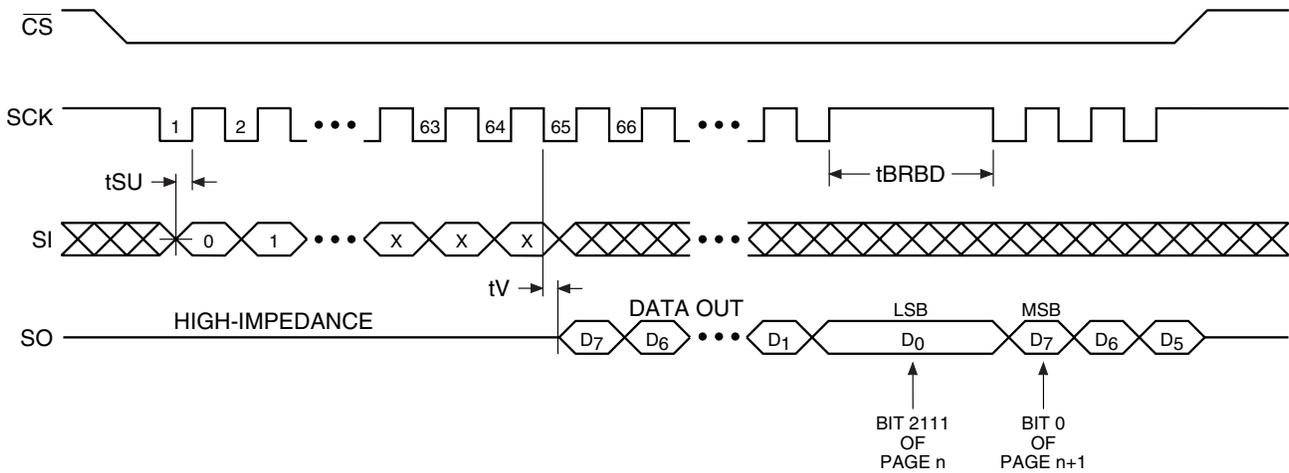
Detailed Bit-level Read Timing – Inactive Clock Polarity High (Continued)
