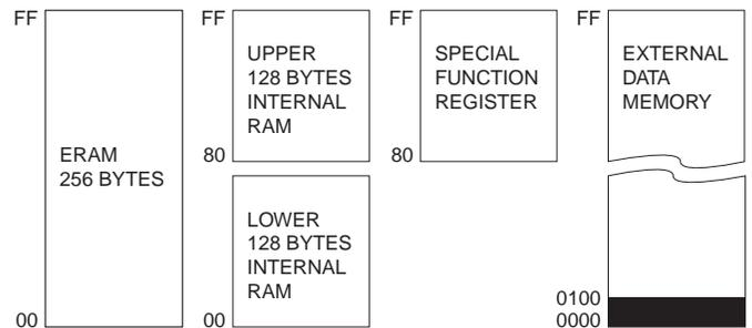
With EXTRAM = 0, the ERAM is indirectly addressed, using the MOVX instruction in combination with any of the registers R0, R1 of the selected bank or DPTR. An access to ERAM will not affect ports P0, P2, P3.6 ( $\overline{WR}$ ), and P3.7 ( $\overline{RD}$ ). For example, with EXTRAM = 0,
