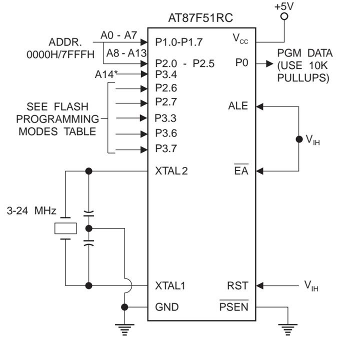
\*Programming address line A14 (P3.4) is not the same as the external memory address line A14 (P2.6).
