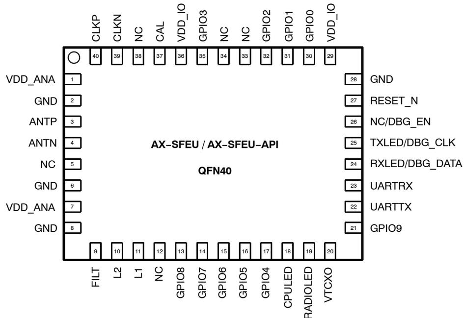
NOTE: Pins 24–26 have different functionalities in AT command and API versions, so for these pins AX-SFEU/AX-SFEU-API explanations are shown respectively.
