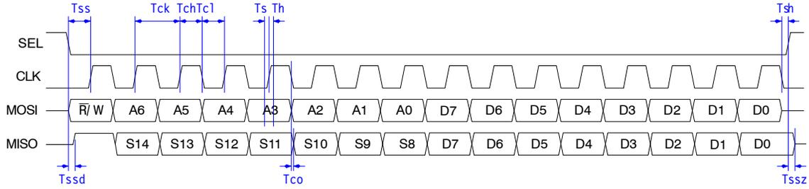
Figure 6. SPI 8 Bit Read/Write Access with Timing
