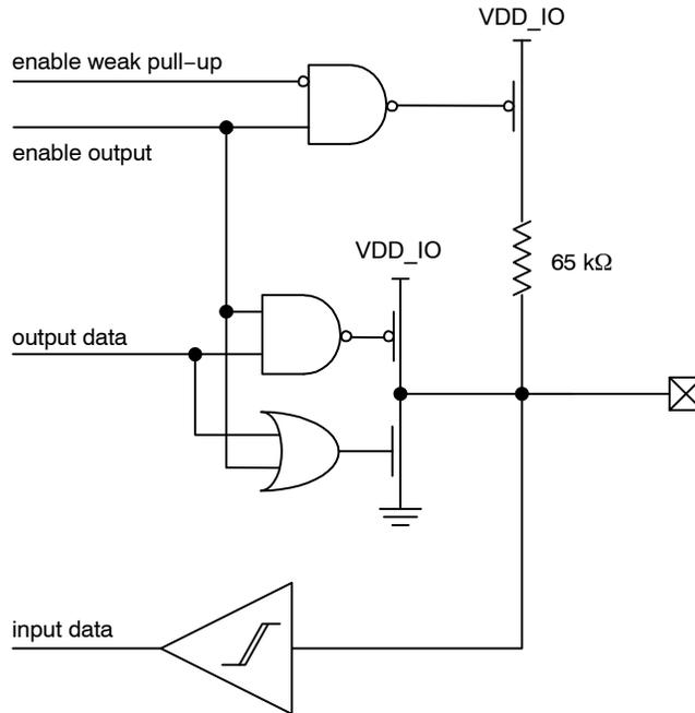
Figure 5. GPIO Pin
