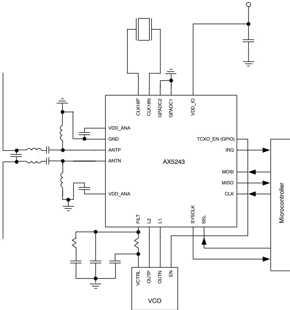
Figure 13. Typical Application Diagram with External VCO
