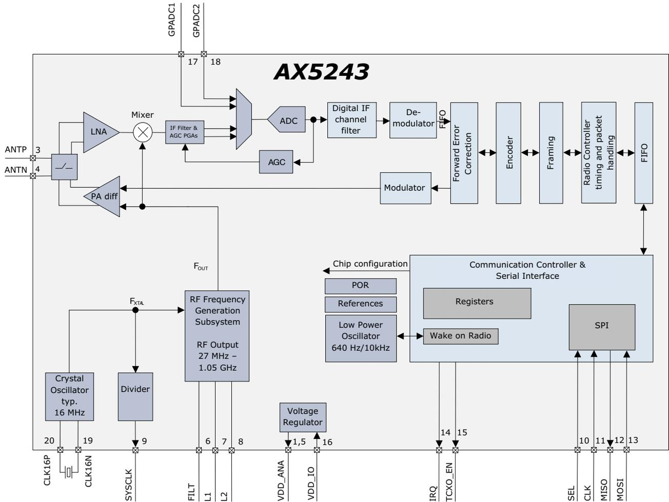
Figure 1. Functional Block Diagram of the AX5243
