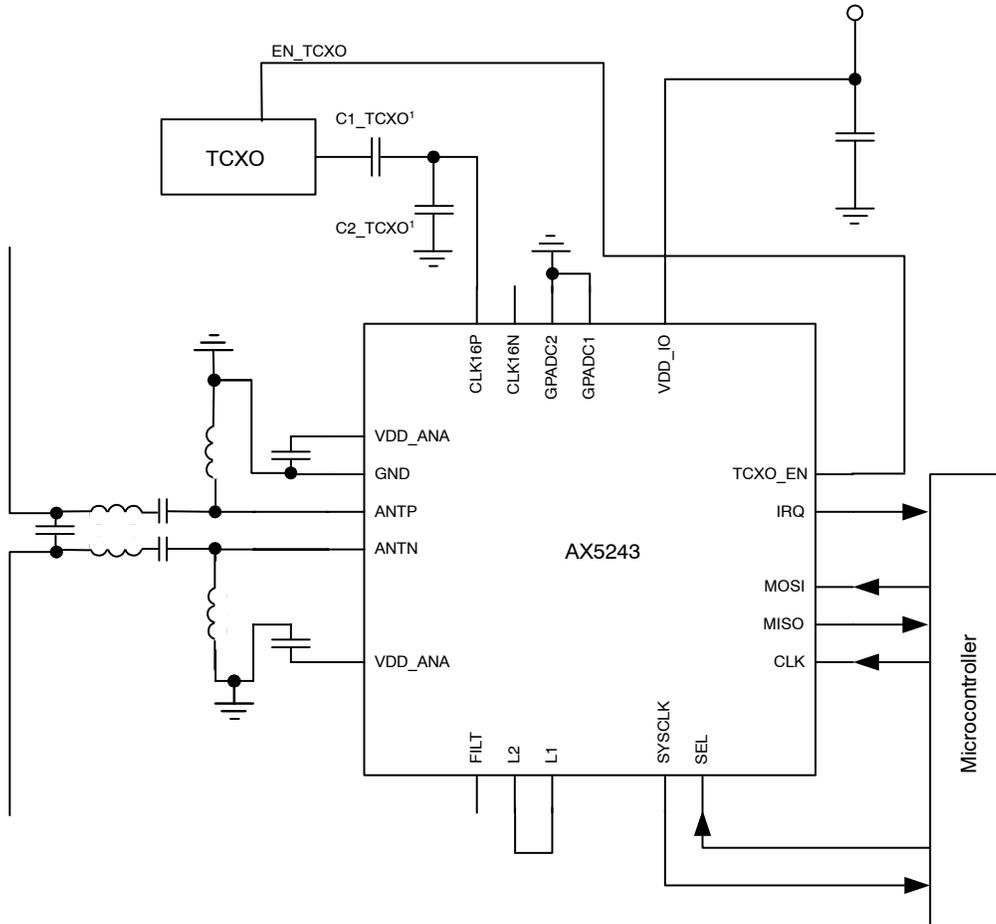
Note 1: For detailed TCXO network recommendations depending on TCXO output swing refer to the AX5243 Application Note: Use with a TCXO Reference Clock.
