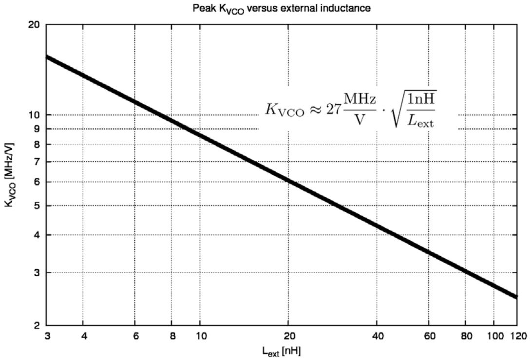
Figure 4. VCO with External Inductors: Typical K<sub>VCO</sub> vs. L<sub>ext</sub>
