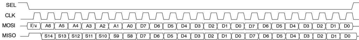
Figure 8. SPI 16 Bit Long Read/Write Access
