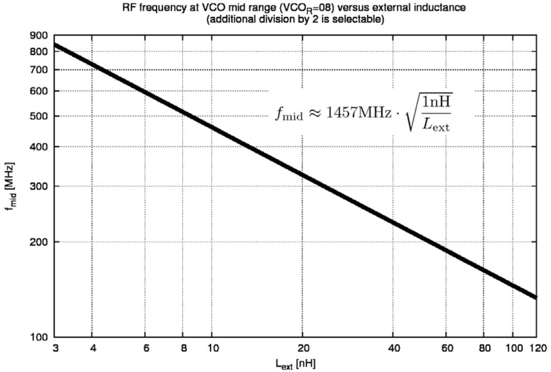
Figure 3. VCO with External Inductors: Typical Frequency vs. L<sub>ext</sub>
