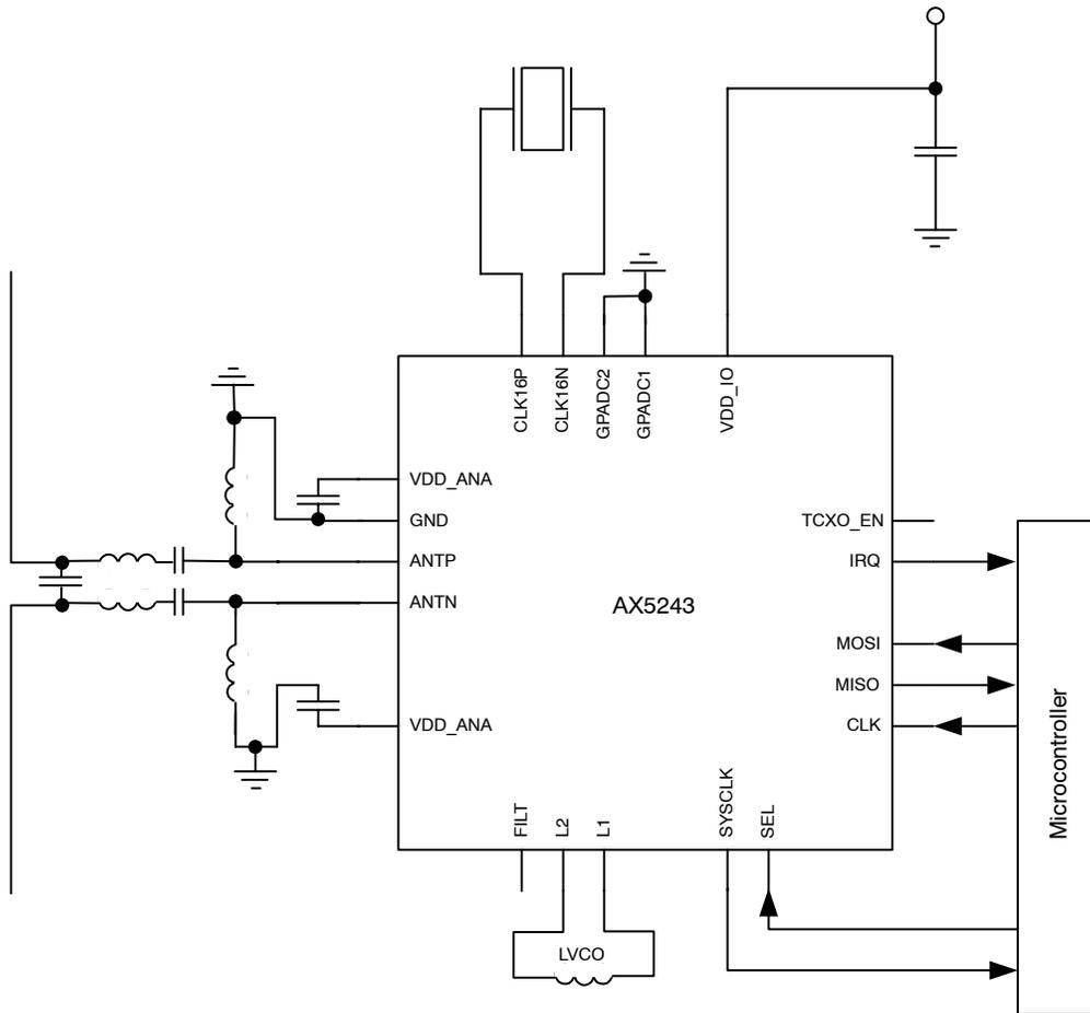
Figure 12. Typical Application Diagram with External VCO Inductor
