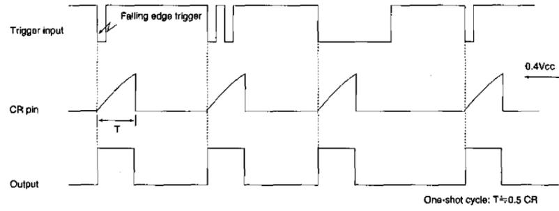
Fig. 10 Basic operation timing chart (Falling edge trigger)
