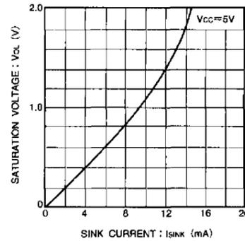
Fig. 3 Output voltage (logic 0 side) characteristic
