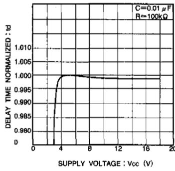
Fig. 4 Power supply voltage - delay time characteristic
