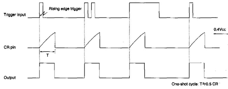
Fig. 9 Basic operation timing chart (Rising edge trigger)
