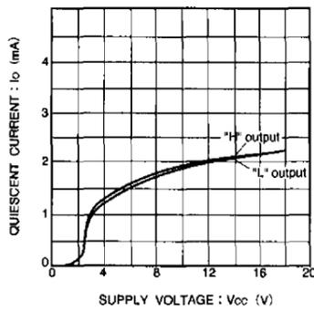
Fig. 1 Quiescent current - power supply voltage characteristic
