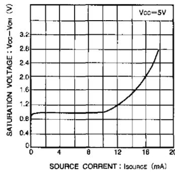
Fig. 2 Output voltage (logic 1 side) characteristic
