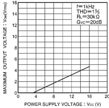
Fig. 5 Maximum output voltage vs. power supply voltage
