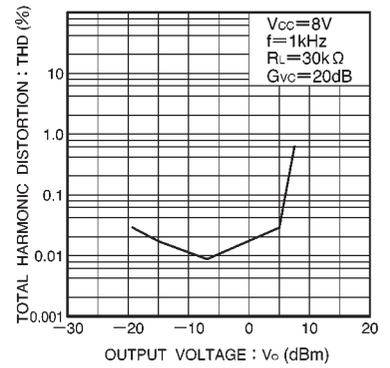
Fig. 6 Total harmonic distortion vs. output voltage
