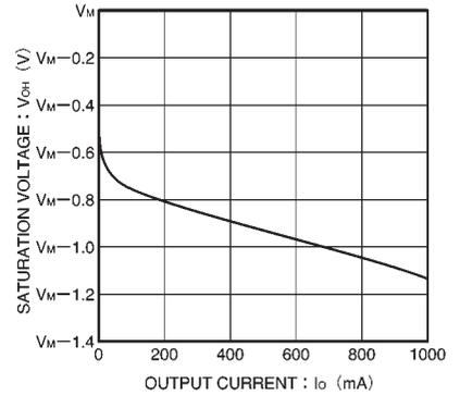
Fig.19 Upper-side output saturation voltage vs. output current
