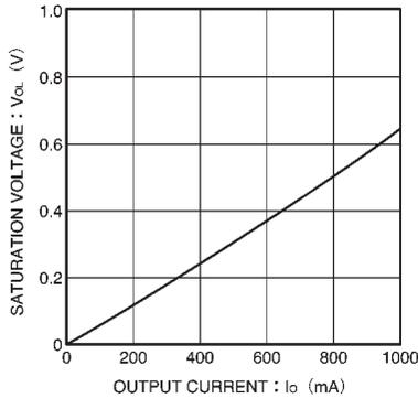
Fig.20 Lower-side output saturation voltage vs. output current
