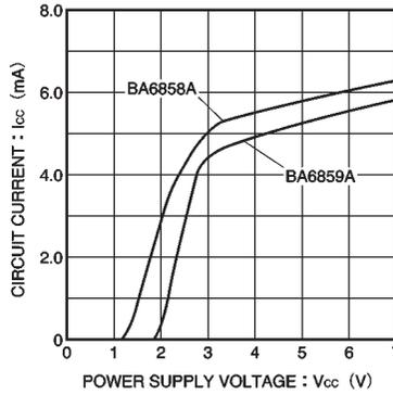
Fig.18 Power supply current vs. power supply voltage
