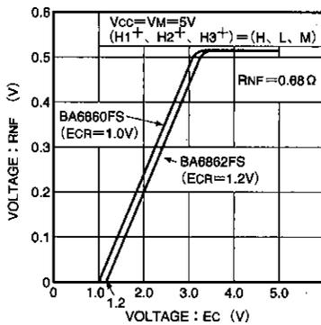
Fig.6 RNF voltage vs. Ec voltage
