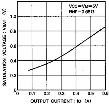
Fig.9 Low-side output saturation voltage vs. output current
