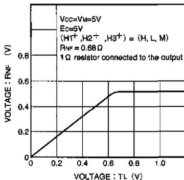
Fig.7 RNF voltage vs. TL voltage
