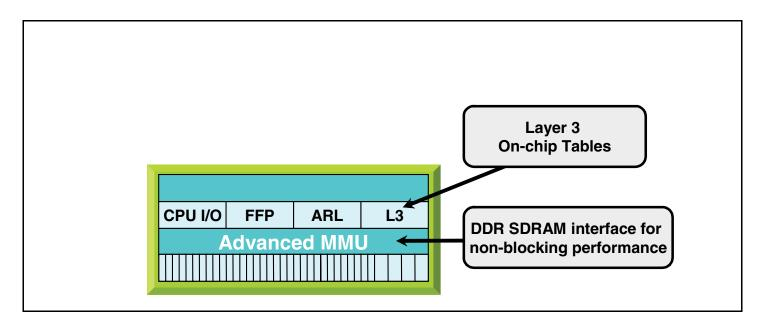
The BCM5655 network switch is the most advanced multi-layer, single chip solution for high density  $48 \times 10/100$  Mbps ports and  $4 \times 10/100/100$  Mbps Ethernet uplinks.
