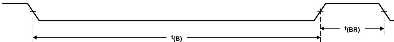
Figure 1. Break Timing
