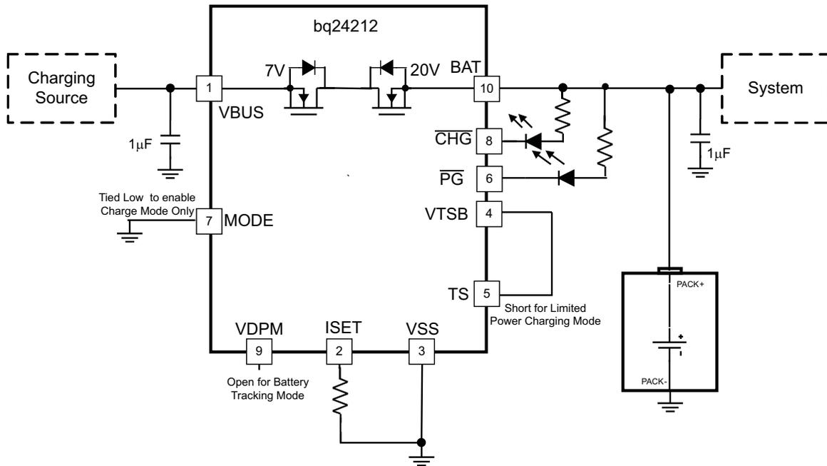
Figure 2. Typical System Schematic for Solar Charger Application
