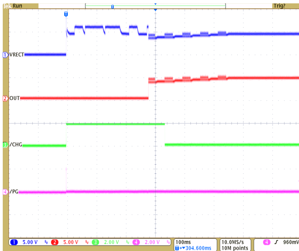
Figure 3. Power-Up In a Wireless Power Application
