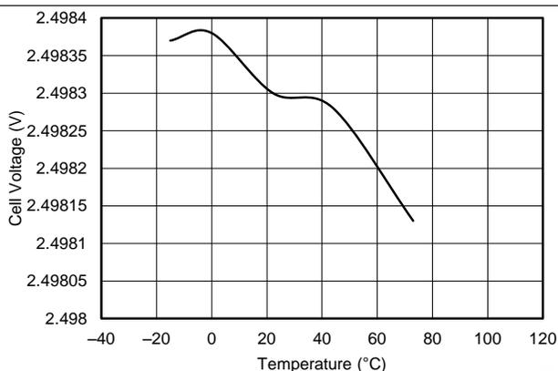
Figure 17.  $V_{CELL}$  Measurement at 2.5-V vs. Temperature
